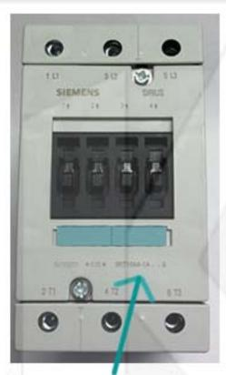
The contactor part number is found on the front on the contactor
