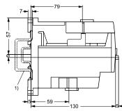
1) For mounting on 35 mm standard mounting rail (15 mm deep) acc. to EN 50 022 or 75 mm standard mounting rail acc. to EN 50023
