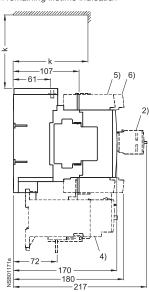
Clearance from earthed parts with directly mounted overload relay: lateral: 10 mm front: 20 mm
